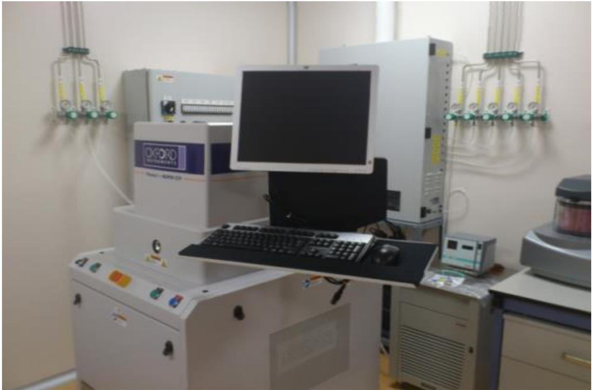
Figure 4.5-2 DRIE etching system: Oxford Instruments Plasma Pro NGP80ICP65 for Deep Etching.
