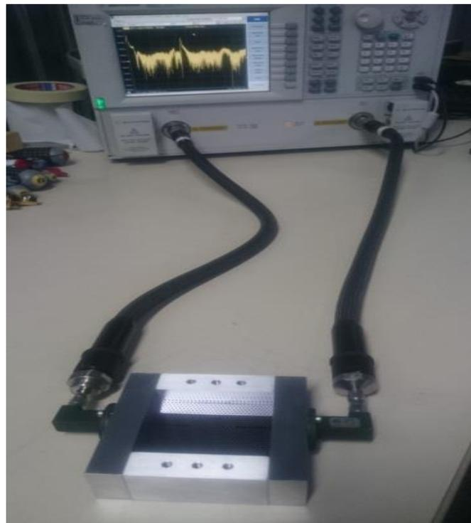
*Figure 4.7-2 Silicon resonator inside of the test-fixture connected to the vector network analyzer.*
