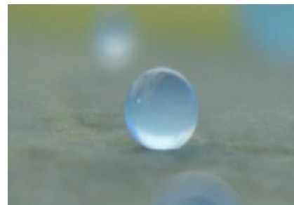
Fig. 4. One of the printed images that was used in order PTs to draw and measure the contact angle by a protractor
