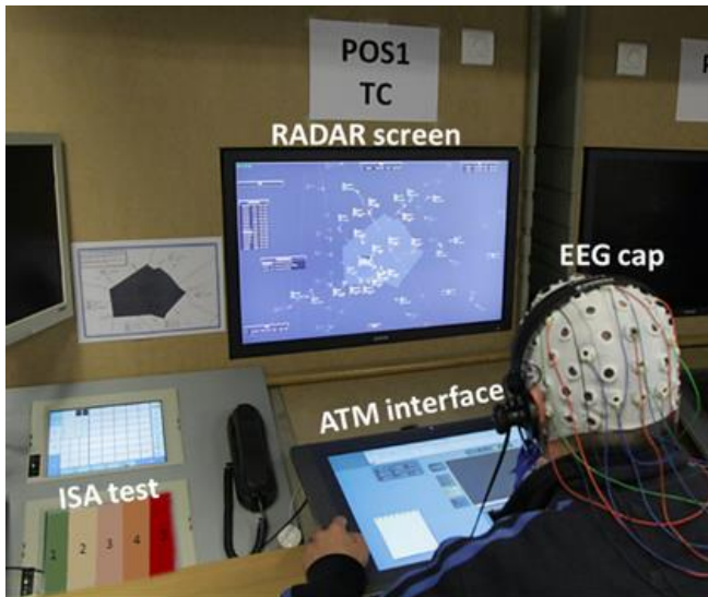
Figure 43. The ENAC simulator platform, composed of two screens, a 30" (RADAR) screen to display radar image and a 21" screen to interact with the radar image (ATM interface). On the little screen on the left bottom, the ISA test was proposed every 3 minutes.
