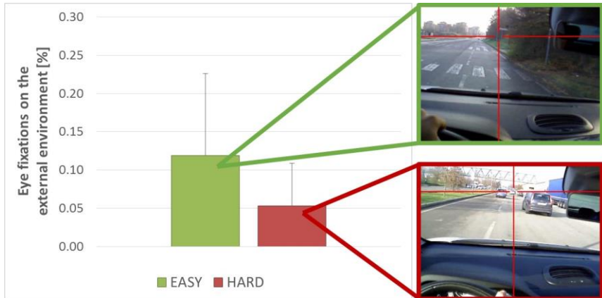
Figure 33. Mean and standard deviation of the eye fixations over the external environments, in other words on all these regions of the scene that do not contain information (e.g. infrastructure, vehicles, signage) useful for the driving. The fixations during the EASY condition (green bar) over the environment were significant higher than during the HARD condition (red bar). For each condition two representative frames are reported on the right: on the top the EASY condition, with the driver's gaze fixed on the external environment; on the bottom the HARD condition, with the driver's gaze fixed on the precedent vehicles.
