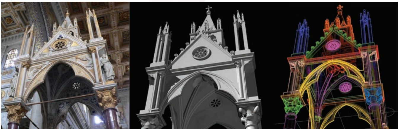
Fig. 2 Rome, San Paolo fuori le Mura, ciborium. Three aspects of architectural relief: chromatic survey using digital photography, morphological survey through the rendering of the geometric model, and decomposition of the object into assembled elements.
