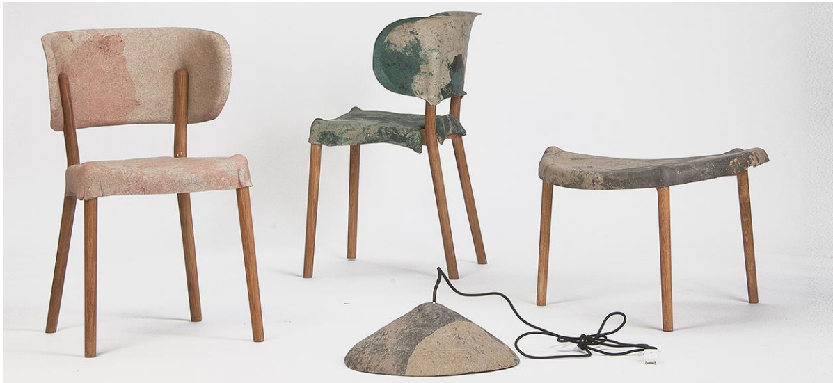
Figure 10. Nikolaj Steenfatt, "Impasto" a biodegradable natural fibre composite made of leftovers from wood, coffee and skin production.
