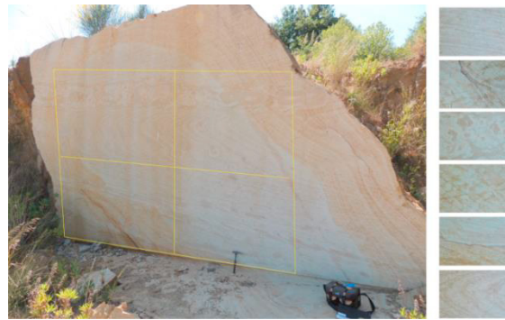
Fig. 8. An example of the varieties (each of which corresponds to a sedimentary facies), that can be produced by a rational use of the blocks (highlighted in yellow) which can be extracted in the sector C of the quarry
