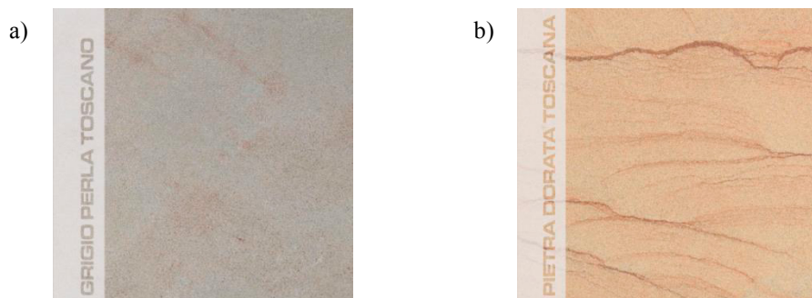
Fig. 2. Commercial variants of the Manciano Sandstone in the Gamberaio quarry: (a) Grigio Perla Toscano® ; (b) Pietra Dorata® with distinctive Liesegang rings
