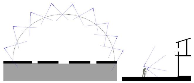
Fig. 10: Shooting with converging axes
