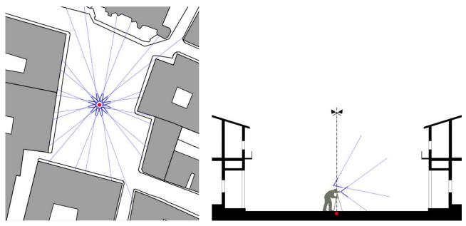
Fig. 11: Panoramic shooting (cylindrical, spherical or partial)
