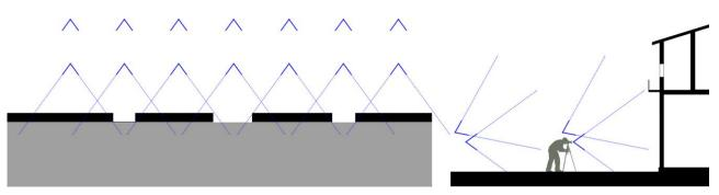
Fig. 9: Shooting with parallel axes (simple or multiple)
