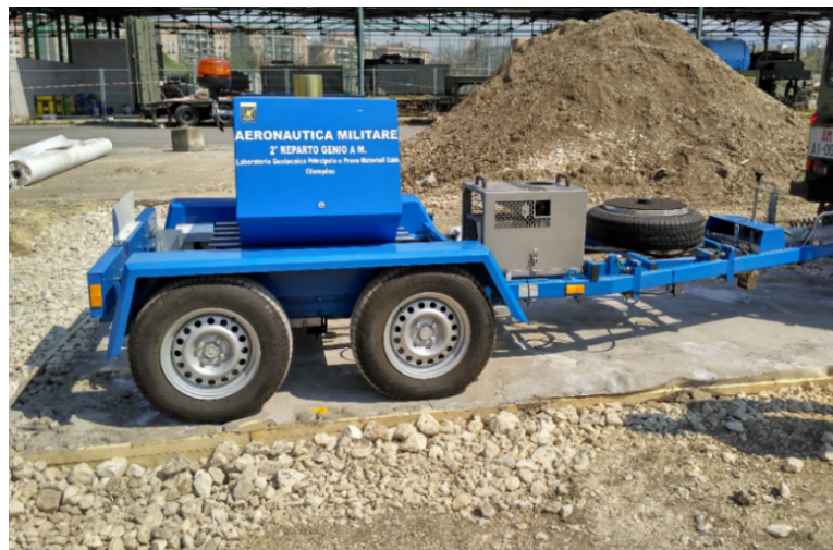
Figure 15. The HWD machine over the M4-treated area.
