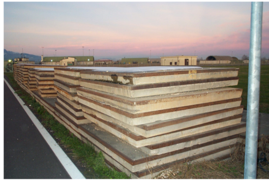
Figure 2. Precast concrete slabs with a steel containment profile.
