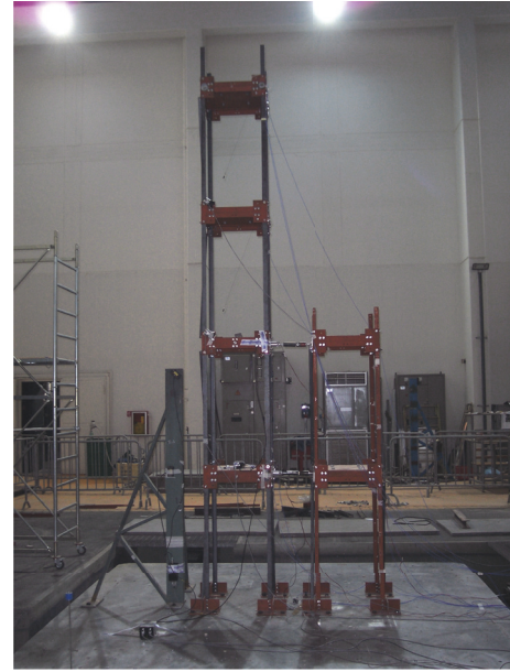
FIGURE 1: Tridimensional physical model mounted on the shaking table with MR damper at the second story.
