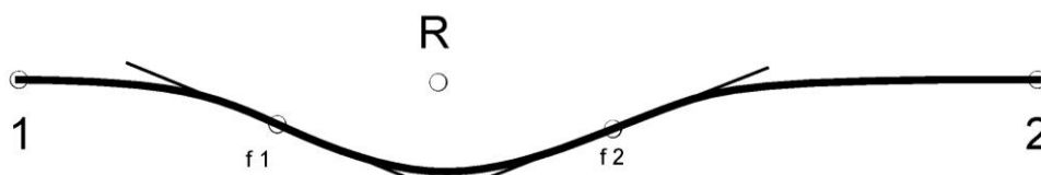
Figure 2. The point attractor A inflects the linear trajectory of the shortest path determining inflection points f1 and f2.
