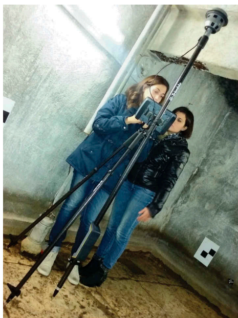
Figure 2. The Trimble V10 terrestrial imaging system: configuration for integration with total stations; on the right the visual field generated by the disposition of the cameras.
