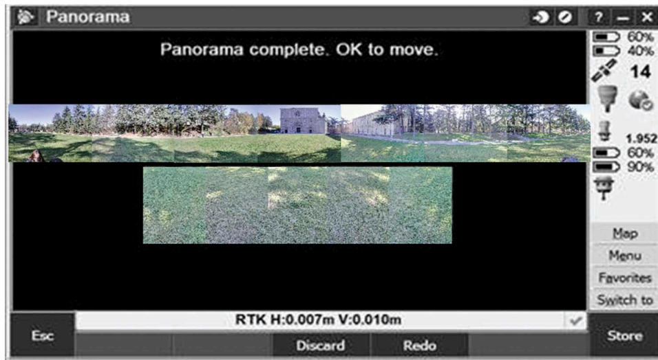
Figure 3. Screen of the controller during the acquisitions effectuated with the imaging rover (IR).
