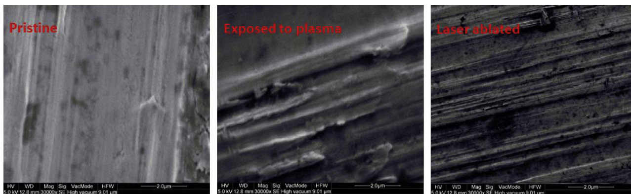
Fig. 3. SEM images of pristine, plasma exposed, and laser ablated Tantalum.
