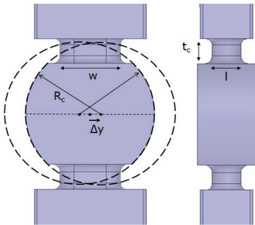
Figure 2: Sketch of the front view (left) and lateral view (right) of the input/output coupler.
