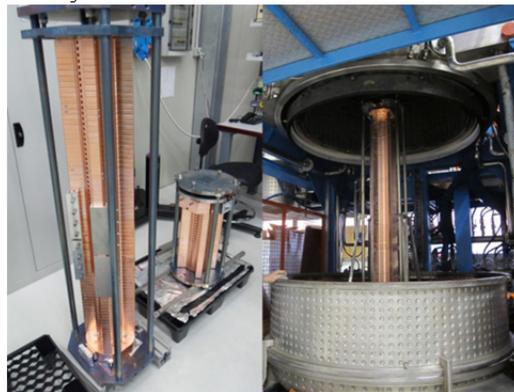
Figure 4: (Left) two half structures before brazing; (right) full assembled structure in the LNL-INFN oven.
