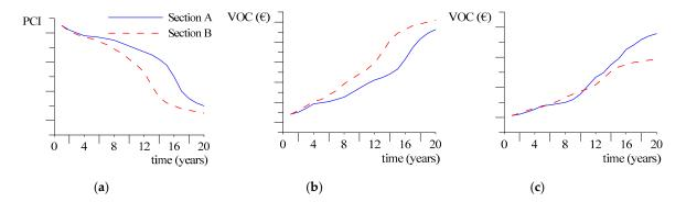
**Figure 2.** Comparative of traffic influence on VOC: (a) pavement condition performance of sections A and B; (b) VOC section A and section B, where traffic at section A is equal to traffic at section B; and (c) VOC section A and section B, where traffic at section A is higher than traffic at section B.
