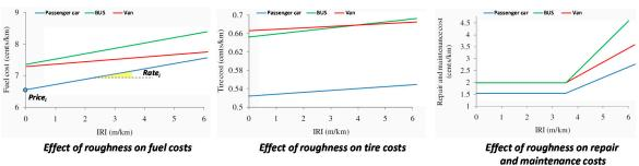
Figure 8. Diagrams to evaluate the effect of roughness on VOC.
