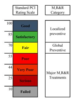
Figure 5. PCI rating scale.
