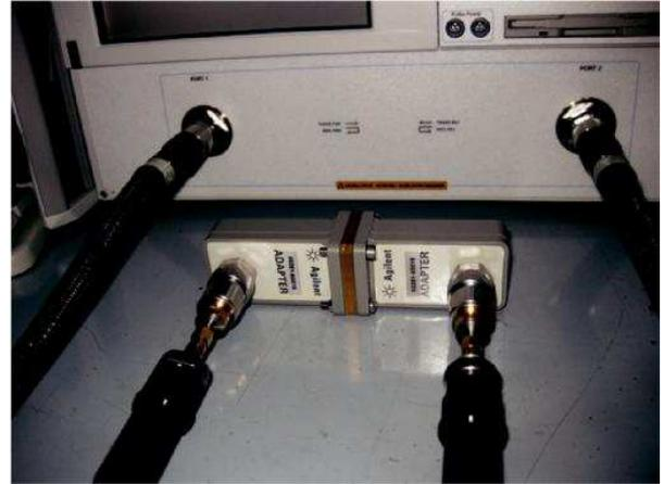
Figura 9-2 Set-up sperimentali: in guida WR430 (a); in guida WR90 (b).
