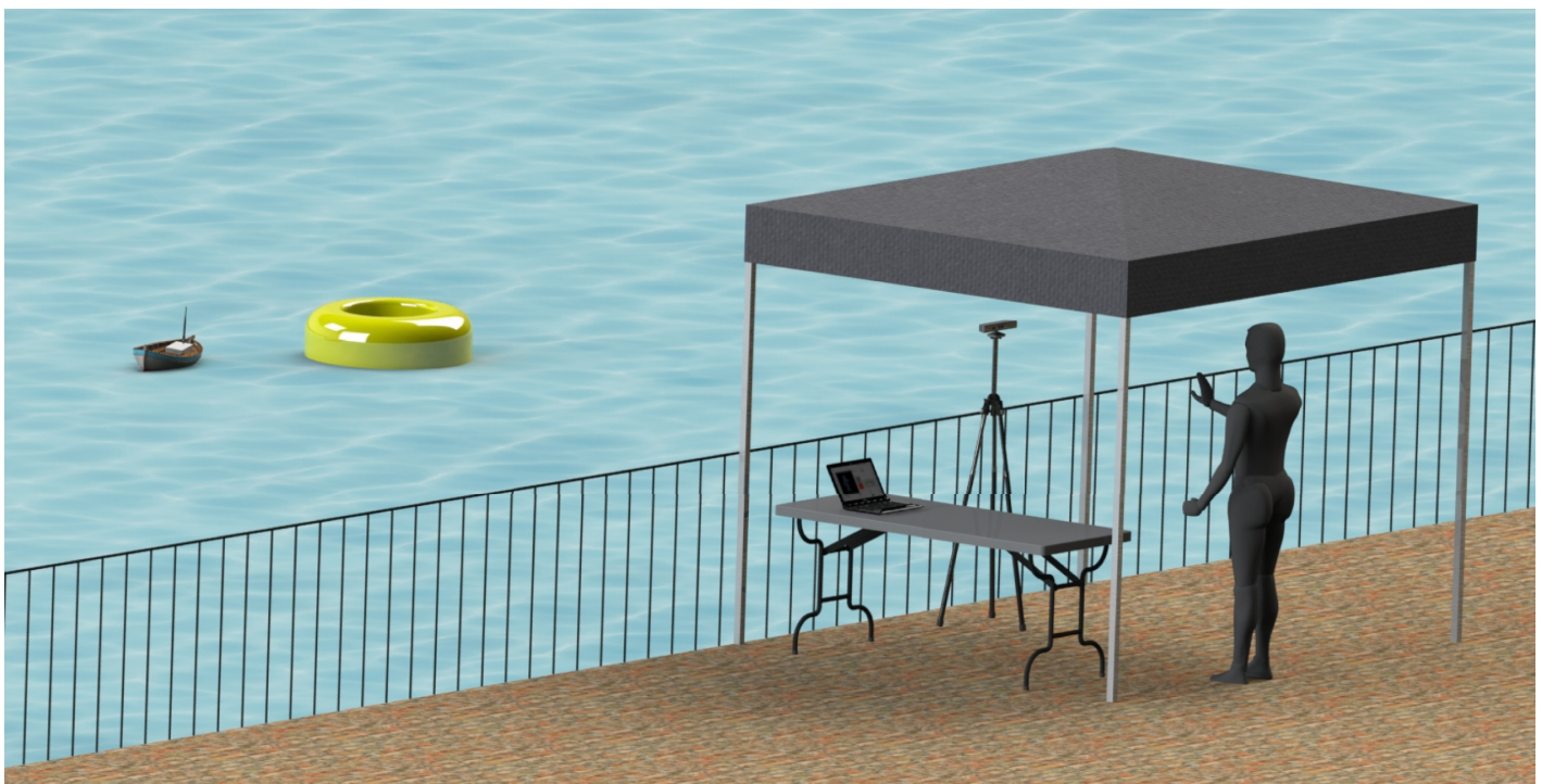
Fig 1. Schematic of the experimental setup. The participant performed the trial on the canal bank. A tent reduced the sunlight exposition of the Kinect to reduce artifacts. The gestures captured by the Kinect were processed in real time by the software running on a laptop and the corresponding commands were sent to the boat via a radio connection. At the same time, water quality data were transmitted from the boat to the laptop.
