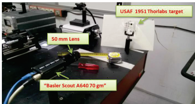
Figure 4: Test-bench with a 50mm microscope lens mounted on a Basler camera.
