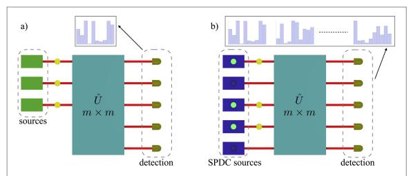
**Figure 1.** (a) Conventional Boson Sampling: the linear transformation is sampled with n sources, injecting a fixed input state for each run. (b) Scattershot Boson Sampling: m SPDC sources are connected in parallel to the m ports of a linear transformation. Each event is sampled from a random (though known) input state.
