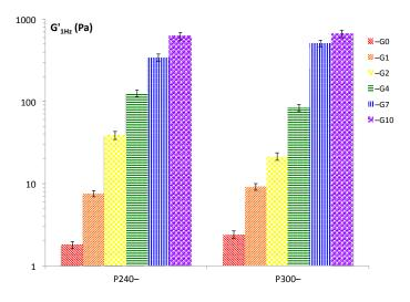
**Figure 3.** Storage Modulus, G', obtained by means of frequency sweep experiments (25 °C, 1 Hz) for the different hybrid gels. The data are reported as the mean value (n = 3).
