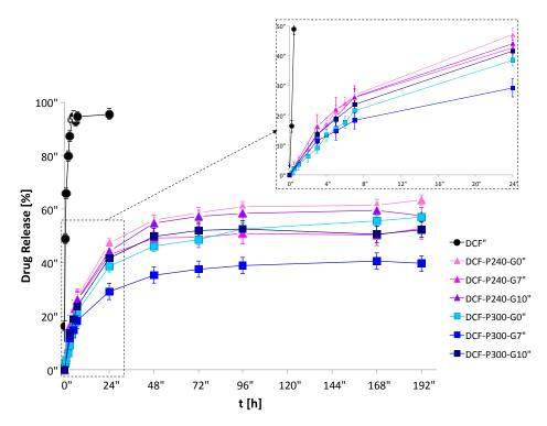
**Figure 5.** Release profiles of free DCF, DCF-loaded within the liposomes and DCF-loaded within the hybrid gels. Results were obtained through dialysis in water at 37 °C. Curves represent the release of DCF from: water solution, as control (black), P240 hybrid gels (P240-G0, P240-G7, and P240-G10 light pink, pink, and purple, respectively), and P300 hybrid gels (P300-G0, P300-G7, and P300-G10 light blue, blue, and dark blue, respectively).
