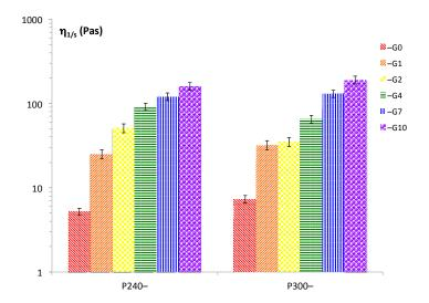
**Figure 2.** Viscosities of P90G/GeCH mixtures, obtained at 25 °C, 1 s<sup>-1</sup>, for the P90G and GeCH systems, at various concentrations (240–300 mg/g and 0–10 mg/mL, respectively). Results are reported as the mean value (n = 3).
