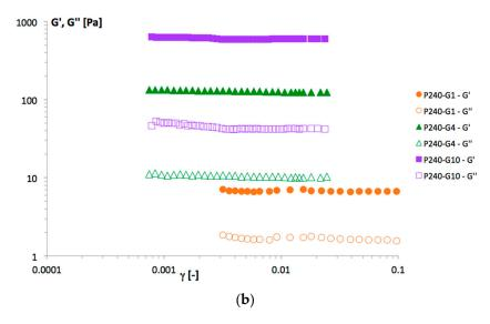
**Figure 4.** (a) Representative mechanical spectra ( $T = 25 \degree$ C) and (b) strain sweep experiments ( $T = 25 \degree$ C) for hybrid gels prepared with different GeCH concentrations: P240-G1 (in orange), P240-G4 (in green), and P240-G10 (in purple). G': full symbols; G'': empty symbols. The tests were performed in triplicate, and standard deviations always laid within 10% of the mean.
