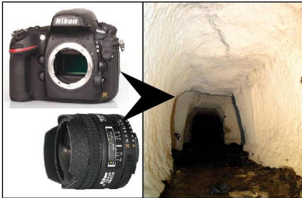
Figure 2. On the left is shown the Nikon D800E and fisheyes lens adopted: Nikkor 16mm, on the right a generic frame recorded during the survey.
