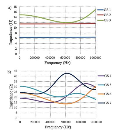
**Figure 6.** Grounding system impedance *vs.* frequency (no soil ionization): (a) Concentrated grounding systems; (b) Spatially extended grounding systems.
