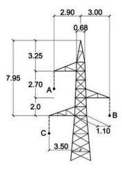
Figure 4. OHL tower head (dimensions in m; the tower height is 31.1 m).
