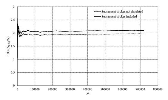
**Figure 8.** 100·  $(N_{BFO}/N)$  ratio vs. N calculated by the Monte Carlo procedure for GS 6 grounding system.
