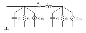
Figure 5. Pi-circuit model.
