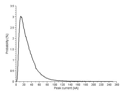
Figure 7. Peak current distribution of lightning strokes impinging on the line.
