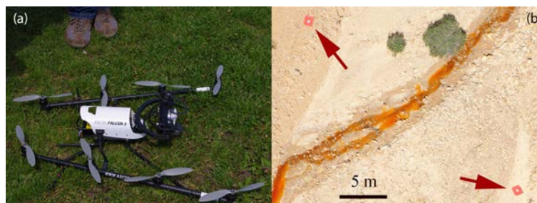
Figure 4. (a) The Astec Falcon 8 UAV and (b) carpets with reflectors used as GCPs for exterior orientation.
