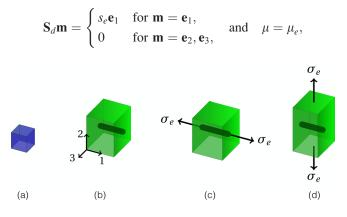
FIG. 6. From left to right: (a) dry state; (b) free–swollen state:  $\sigma_e = 0$ , and  $\mu_e = -10 \text{ J/mol}$ ; (c) swollen with traction along the fiber:  $\sigma_e = 50 \text{ kPa}$ , and  $\mu_e = -10 \text{ J/mol}$ ; (d) swollen with traction orthogonal to the fiber:  $\sigma_e = 50 \text{ kPa}$ , and  $\mu_e = -10 \text{ J/mol}$ .
