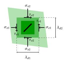
FIG. 10. Sketch of the plane section of unit normal  $\mathbf{e}_3$  of the unit cube at the dry state (dark green square), at the free–swelling state (light green diamond), and at the constrained state (green rectangle).
