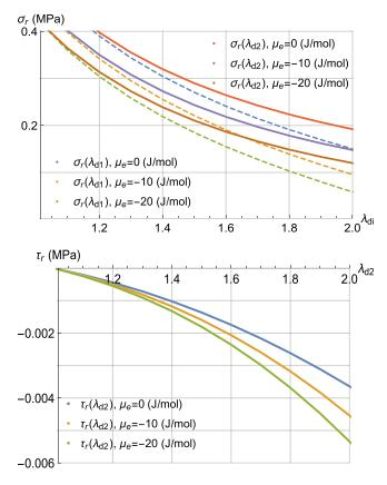
FIG. 11. Normal stroke curves  $\sigma_r(\lambda_{d1})$  at  $\lambda_{d2} = 1$  and  $\sigma_r(\lambda_{d2})$  at  $\lambda_{d1} = 1$  and tangential stroke curves  $\tau_r(\lambda_{d2})$  at  $\lambda_{d1} = 1$  at different values of  $\mu_e$ , being G = 0.1 MPa and  $\gamma = 0.1$ .
