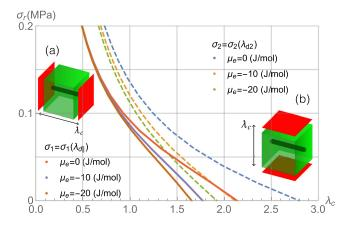
FIG. 9. Stroke curves  $\sigma_r(\lambda_c)$  for different values of  $\mu_e$ : case a)  $-\sigma_1(\lambda_{d\parallel})$  (solid lines); case b)  $-\sigma_2(\lambda_{d2})$  (dashed lines). The insets show the constraints (red surfaces) acting on the fibered gel cube in the two cases (a) (left) and (b) (right).
