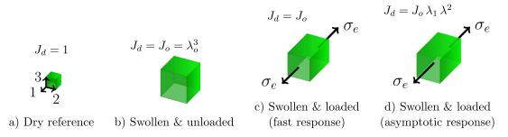
FIG. 3. From left to right: (a) dry state; (b) free-swollen state; (c) fast response state under swelling and loading; (d) asymptotic state under swelling and loading. For a gel with G = 0.1 MPa,  $RT/\Omega = 40$  MPa,  $\chi = 0.2$ , under a traction  $\sigma_e = 0.1$  MPa, we have:  $J_o = 18.5$ ,  $J_d \simeq 23$ . Plots are in scale.
