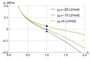
FIG. 5. Stress–stroke curves  $\sigma_r = -\sigma_e(\lambda_1)$  at different values of  $\mu_e$  when  $\mu_o = -10$  J/mol and  $\lambda_o = 2$ , being G = 0.1 MPa.
