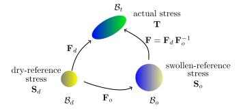
FIG. 1. Given a dry ball  $\mathcal{B}_d$ , the swollen and stress-free state  $\mathcal{B}_o$  only differs for a change in size, whereas the actual state  $\mathcal{B}_t$  for a change in size and possibly in shape.
