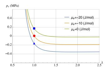
FIG. 2. Pressure–stroke curves  $p_e(\lambda, \mu_e, \lambda_o)$  for three values of  $\mu_e$  with  $\lambda_o = 2$ , corresponding to  $\mu_o = -10$  J/mol. When  $\mu_e < \mu_o$  ( $\mu_e > \mu_o$ ) the corresponding blocking pressure is determined on the vertical axis  $\lambda = 1$  in correspondence of the blue triangle (square) on the blue (green) curve.
