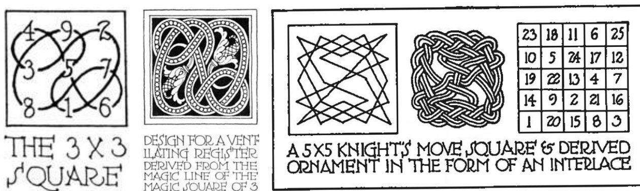
Fig. 5a – 5b. Genesis and final drawing of the ventilation grille in Rochester Chamber of Commerce, in Bragdon Frozen Fountain pag 76
