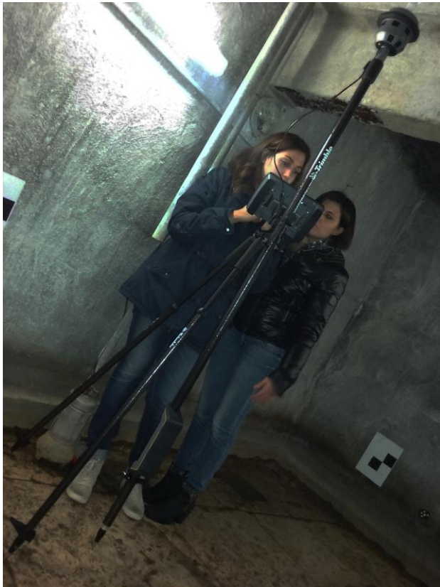
Figure 4. Trimble V10 Imaging Rover equipped with a 360 degrees prism on a topographic rod
