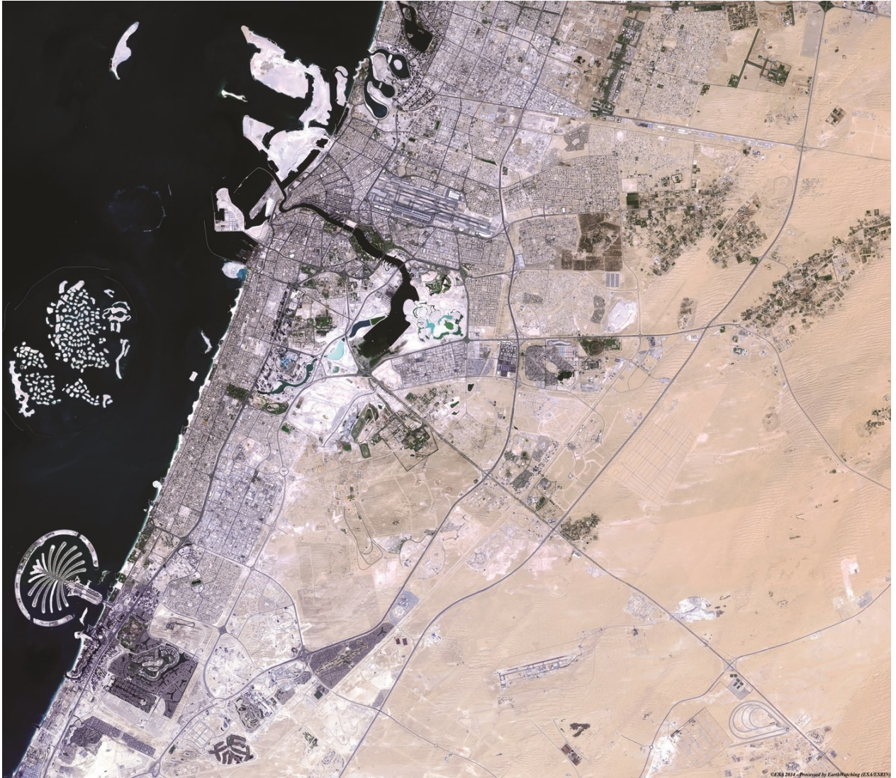
Figure 9. Multispectral satellite image of Dubai Emirate, generated from data acquired by the AVNIR-2 of ALOS spacecraft on 2 November 2010 and visualized in natural colours (RGB 321). Source: JAXA/ESA.
