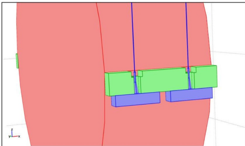
Figure 4.10: design of the lower clamping system on the lateral flat of the mirror: the mirror is in red, fibers with anchors in blue and the ear is in green.
