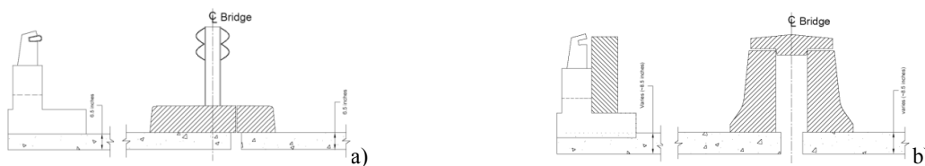
Figure 8-11 a) exterior and interior barrier as Designed in 1965, b) barriers at the time of the collapse
