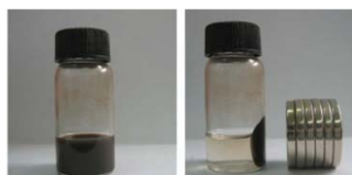
Figure 1-8 Magnetic separation of \text{Fe}_3\text{O}_4 nanoparticles.
