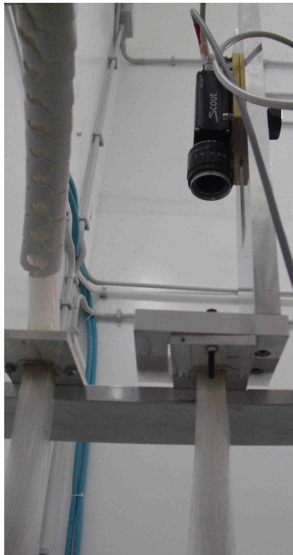
Figure 3.25. The CCD camera based read-out system replaces all the devices used after the fibers, directly detecting the light emitted by the scintillating fibers .
