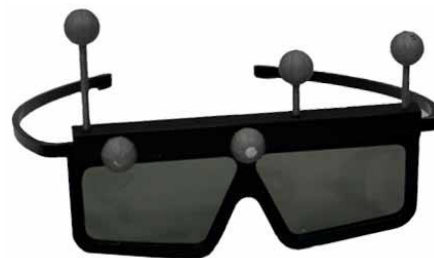
Fig. 12: 3D glasses with IR-camera receivers for tracking the eyes position.
