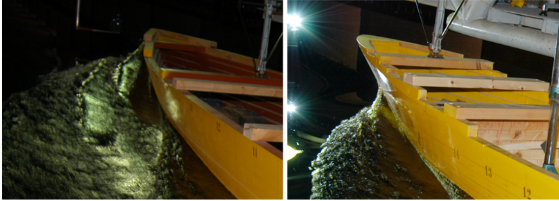
Figure 48: same portion of wave field photographed for the two larger model scales at Fr = 0.35 . Middle scale C.2340 is on the right and large scale C.2469 on the left.
