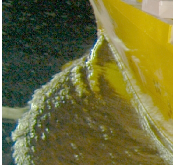
Figure 27: wave pattern of C.2340 at Fr = 0.30 . The bow wave breaking begins clearly to show in its wake the scars generated by the splash up of the crest.
