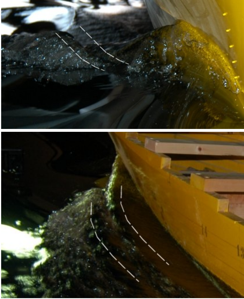
Figure 29: particular of the bow wave of C.2340 at Fr = 0.41 . The secondary splash up is very evident, the scar generated by this splash up is visible in the bottom image.
