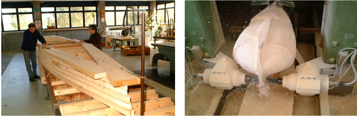
Figure 10: first steps of model construction. Left: wood planks are glued together. Right: numerical milling of the bulb.
