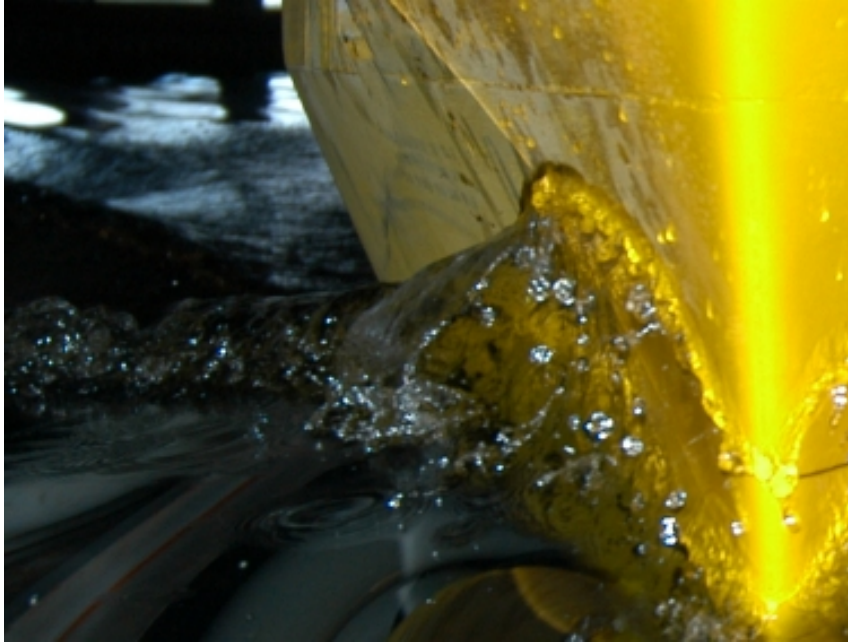
Figure 25: particular of the bow wave of C.2469 at Fr = 0.28 . The first part of the wave is characterized by the formation of drops whereas in the second part the water on the crest turns over and falls down.
