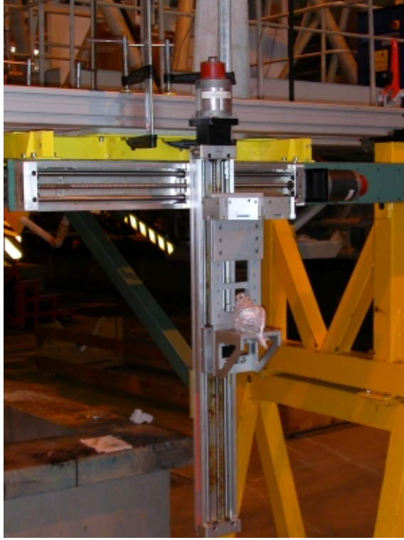
Figure 15: transversal and vertical linear guides mounted on the frame for instrument displacement on the hull's side.
