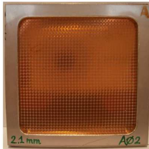
Figure 5.1. The resonant grid employed for reflection and transmission measurements. Geometrical parameters are listed in the text.
