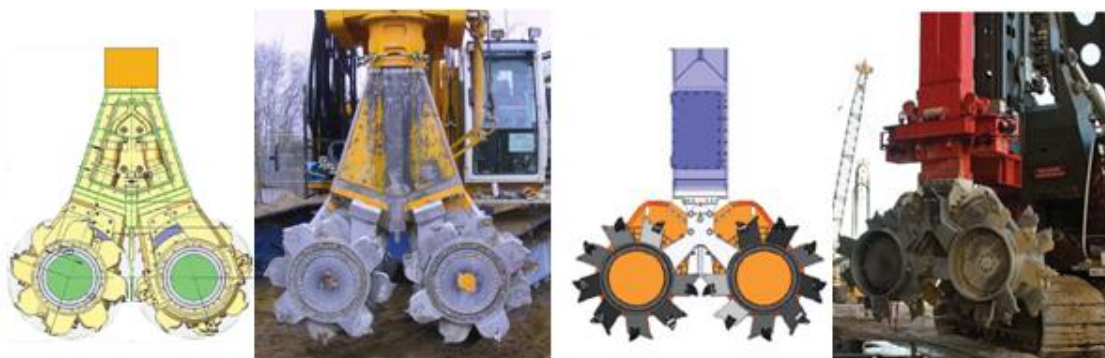
Figura 1.8 - Cutter Soil Mixing, CSM, tecnologia Bauer e Soletanche Bachy (Deschamps 2012).
