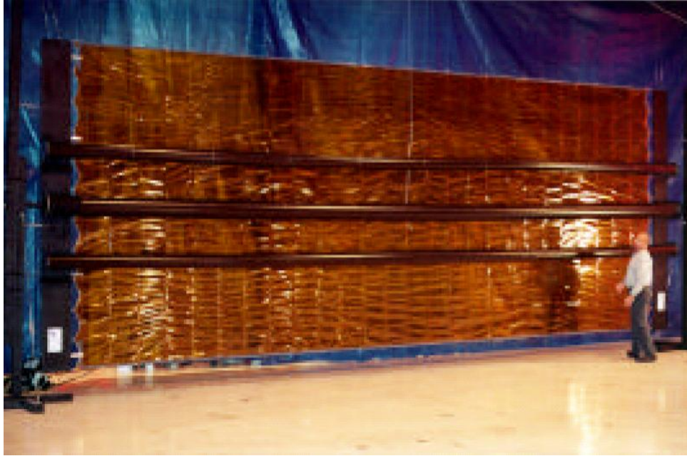
Figure 236: Inflatable Solar Array Prototype
