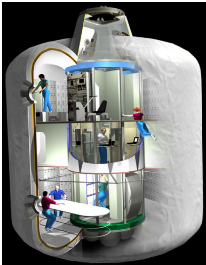
Figure 149: Internal view of TRANSHAB Inflatable Space Module
