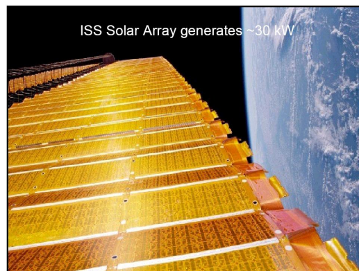
Figure 157: each ISS solar array produces about 30 kW
