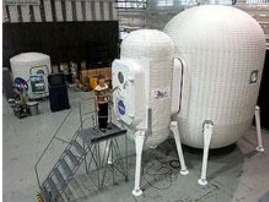
Figure 20: The "planetary surface habitat and airlock unit" has been delivered to NASA Langley for ground-based evaluation of emerging technologies such as health monitoring of flexible structures.
