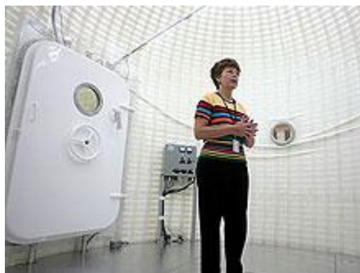
Figure 22: Inflation Structures Project Leader Karen Whitley stands in the center of the 12-foot (3.65 meter) diameter inflatable lunar habitat at NASA Langley Research Center, Hampton, Virginia.
