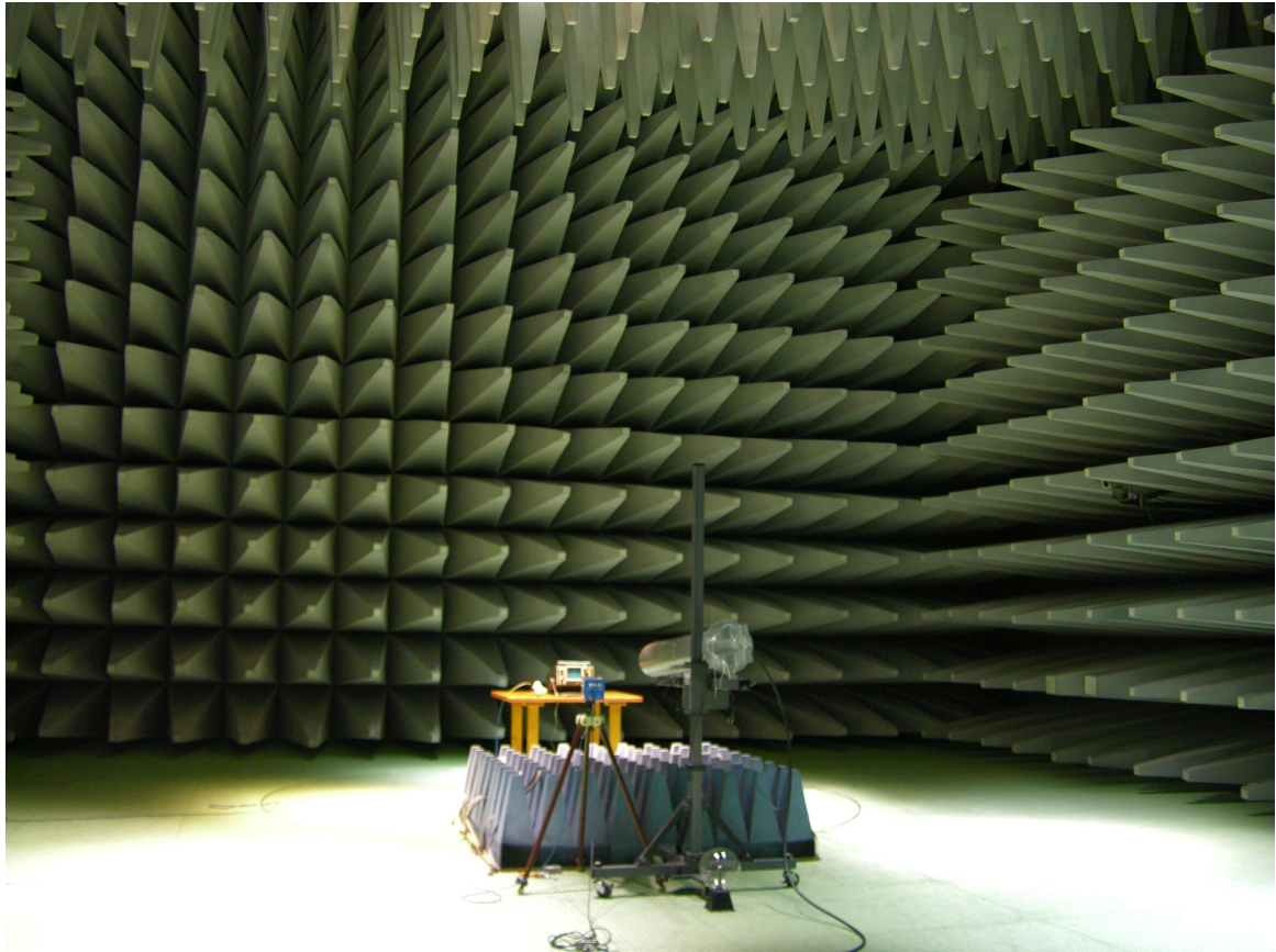
Figure 326: Shielded Anechoic Room (CSA)
