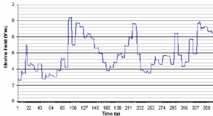
Figure 2.11: Electric field amplitude vs time during one tuner revolution at the frequency of 2 GHz
