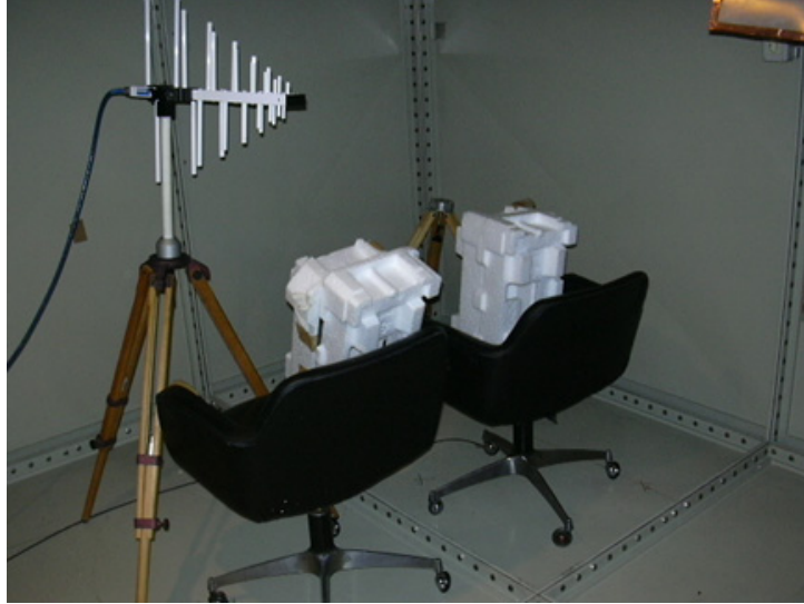
Figure 3.2: Experimental setup with two seats occupied by two “passengers” using a cellular phone.
