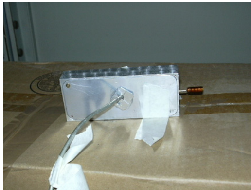
Figure 3.6: The cellular phone mock-up with the antenna tuned at 900 MHz used as a transmitter inside the RC.
