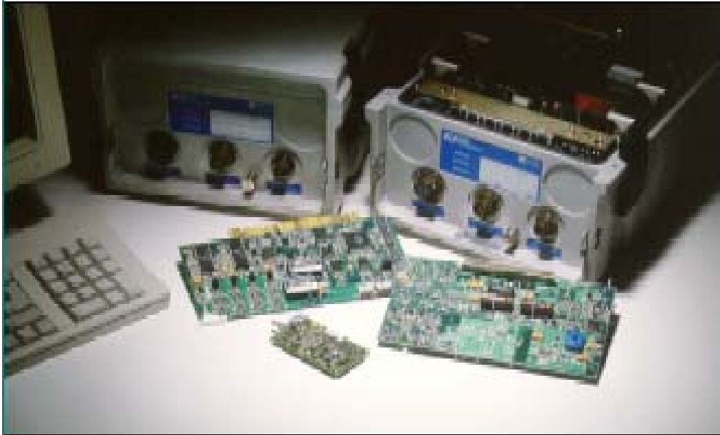
Figure 3.4. Kinematics K2 digital accelerograph ( www.kinematics.com )
