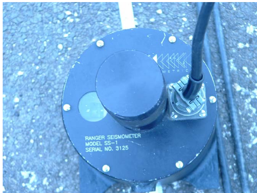
Figure 4.2. Particular of the 1-Hz Kinometrics1 receiver (picture shot from above).
