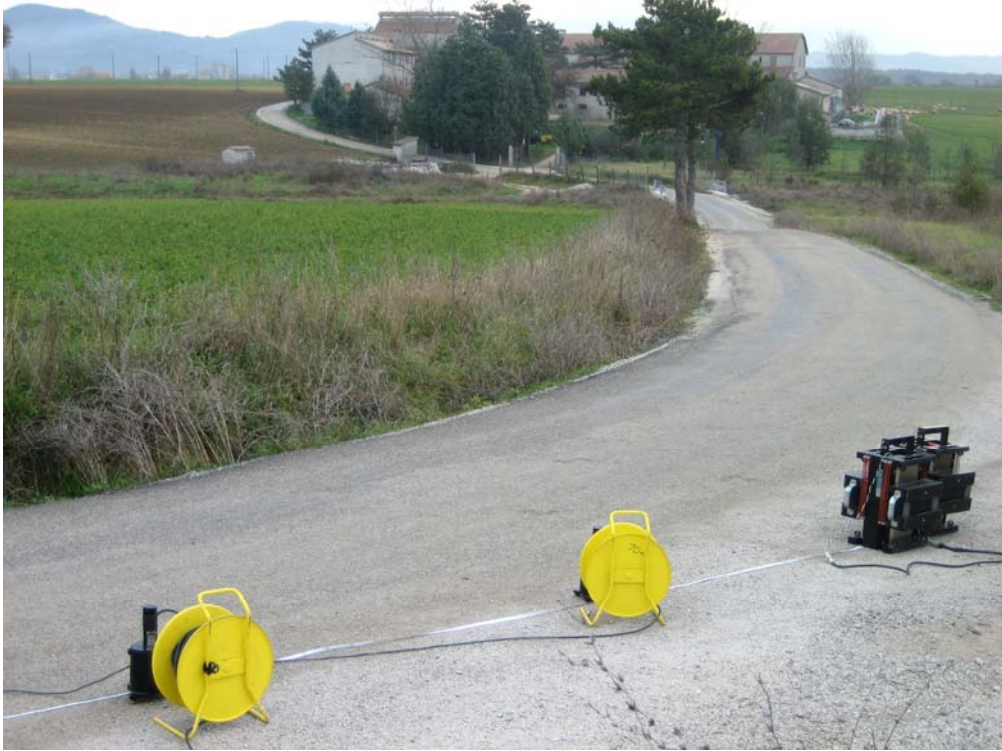
Figure 4.4. Configuration of the USGS surface wave testing system at site 262GBP Gubbio Soil Site Piana (43.314°N,12.59°E) composed of 1-Hz vertical motion sensors and two-100 kg electro-mechanical harmonic wave shakers. The shaker apparatus are arrayed in a parallel circuit and synchronized in phase for controlled swept-sine analysis.
