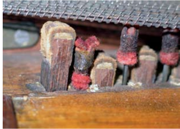
Figure 18. Hammers and dampers of the anonymous square piano in Osaka (College of Music Collection, Osaka).
