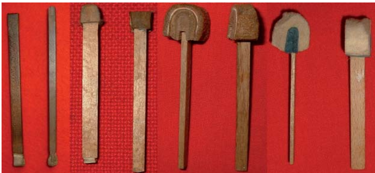
Figure 3. Different types of non-pivoting hammers. From the left: bare hammers ( Tangentenflügel C. F. Schmahl, Regensburg 1791); leathered hammers (anonymous piano, Italy c. 1825); leathered hammers (square piano F. Puglisi, Catania 1849); felt hammers (anonymous square piano, Italy c. 1850).
