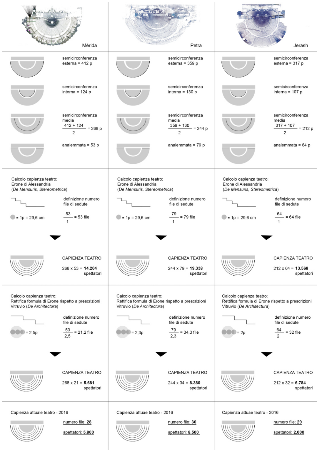
Fig. 9: Comparison between Heron’s rule and the current seating capacity: the theatres in Mérida, Petra and Jerash
