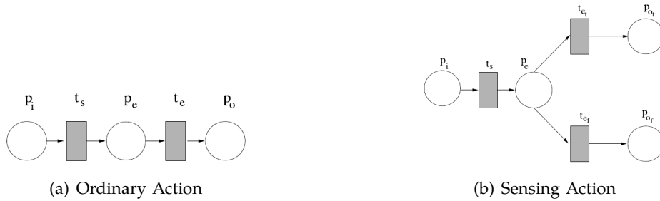
Figure 2.2: Ordinary and sensing actions in a Petri Net Plan
