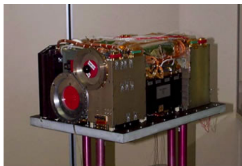
Figure 3.5: The OMEGA instrument in the laboratory. We can see two entrance windows for the visible and the IR channels.
