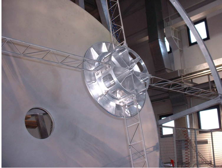
Figure 2.3: Image of the back of the OLIMPO secondary mirror and of the spider that keeps it positioned in front of the primary mirror.
