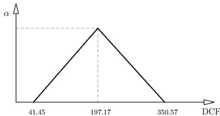
Figure 9. Actual value expressed in the form of a triangular fuzzy number (source: Del Viva 2005)
