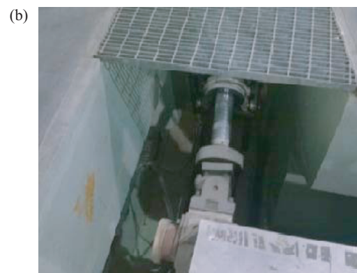
Figure 4.18. Six-degree-of-freedom shaking table in the MAT-QUAL Laboratory of ENEA, “Casaccia” Research Center, Rome. (a) and (b) Details of oil-driven actuators.
