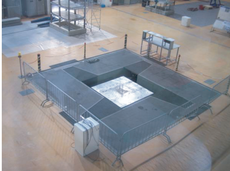
Figure 4.17. Six-degree-of-freedom shaking table in the MAT-QUAL Laboratory (ENEA, “Casaccia” Research Center, Rome).
