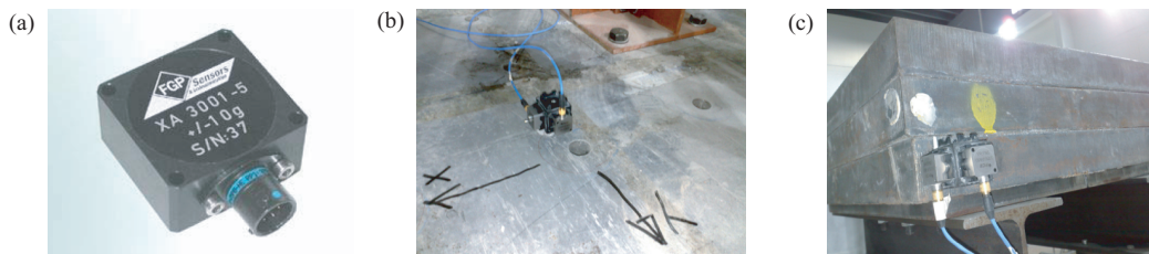
Figure 4.20. Piezotronic PCB piezoelectric accelerometers. (a) Detail of the sensor. (b) Sensors on the shaking table. (c) Sensors on the isolated mass.
