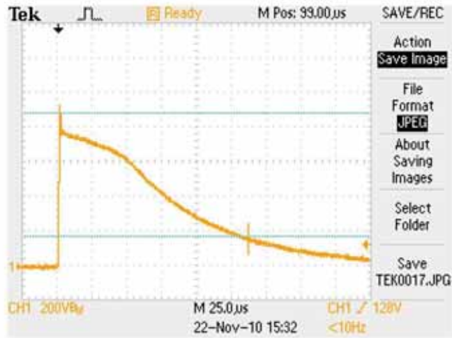
Figure 6.10. Oscillogram of voltage on the SPD terminals (limiting type) under stressing overvoltage of 2,5 kV and wave shape 1,2/50 μs.
