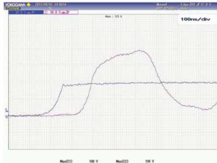
Figure 8.17. Oscillograms of voltage at apparatus to be protected: CH1 voltage on the SPD terminals, CH2 voltage on the load; impulse voltage wave shape 0,25/50 \mu s; U_p = 100 V; resistive load, R = 10^6 \Omega ; line length d = 30 m.
