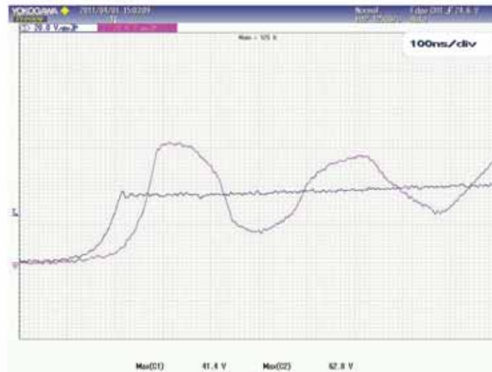
Figure 8.13. Oscillograms of voltage at apparatus to be protected: CH1 voltage on the SPD terminals, CH2 voltage on the load; impulse voltage wave shape 1,2/50 \mu s; Resistive load, R = 10^6 \Omega ; line length d = 15 m.
