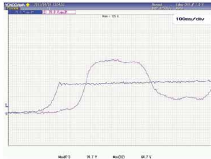
Figure 8.14. Oscillograms of voltage at apparatus to be protected: CH1 voltage on the SPD terminals, CH2 voltage on the load; impulse voltage wave shape 1,2/50 \mu s; Resistive load, R = 10^6 \Omega ; line length d = 30 m.
