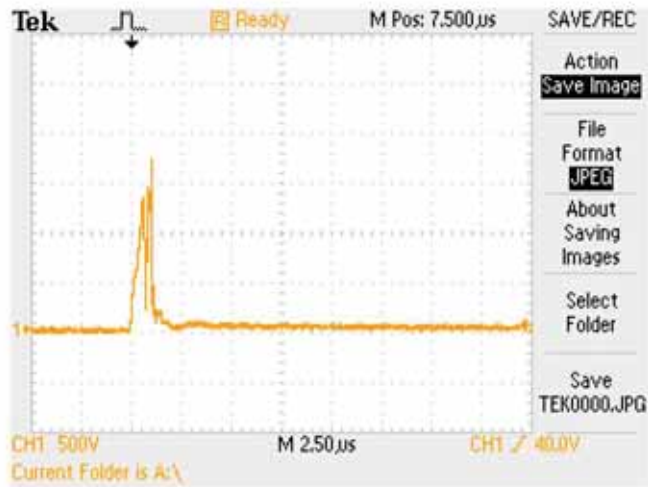
Figure 6.11. Oscillogram of voltage on the SPD terminals (switching type) under stressing overvoltage of 2,5 kV and wave shape 1,2/50 μs.
