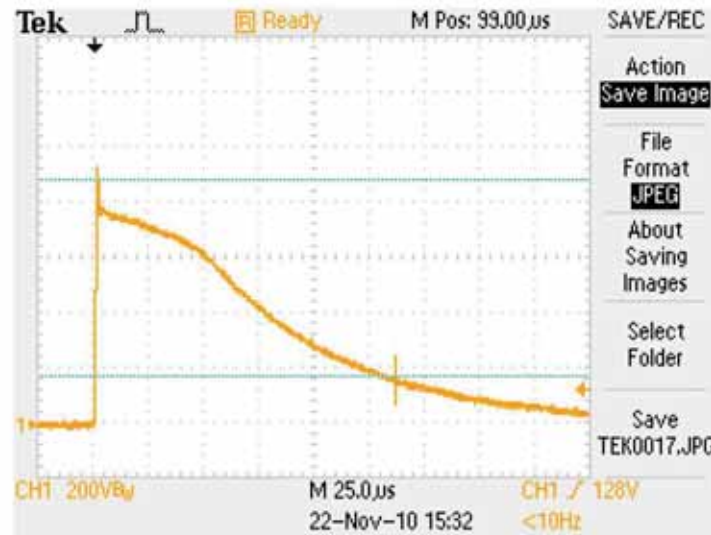
Figure 6.24. Oscillogram of voltage on the SPD terminals (limiting type) under stressing overvoltage of 2,5 kV and wave shape 1,2/50 \mu s.
