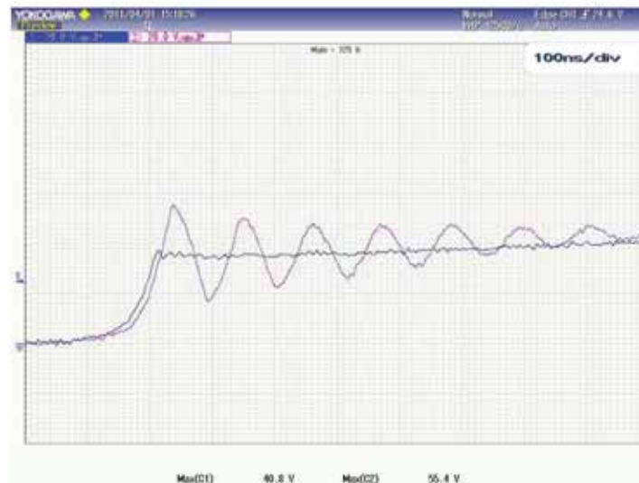
Figure 8.12. Oscillograms of voltage at apparatus to be protected: CH1 voltage on the SPD terminals, CH2 voltage on the load; impulse voltage wave shape 1,2/50 \mu s; Resistive load, R = 10^6 \Omega ; line length d = 5 m.
