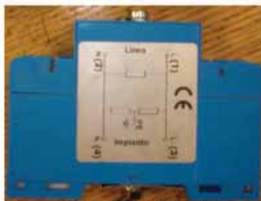
Figure 6.8. Photo of SPD limiting type.
