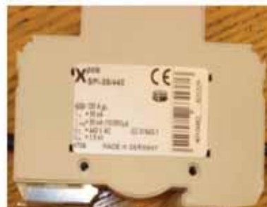
Figure 6.9. Photo of SPD switching type.
