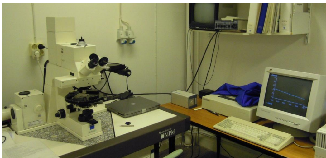
Fig. 3.10. Zeiss MPM800 single beam microscope-spectrometer.
