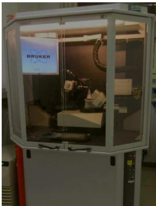
Fig. 3.5. Bruker KAPPA APEX-II single-crystal diffractometer of the Earth Sciences Department, Sapienza University of Rome.
