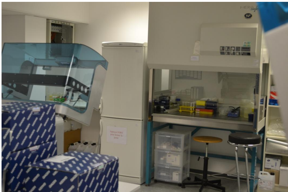
Fig. 2.1.26: safety cabinet for paper point preparation and bacterial lysis before DNA extraction
