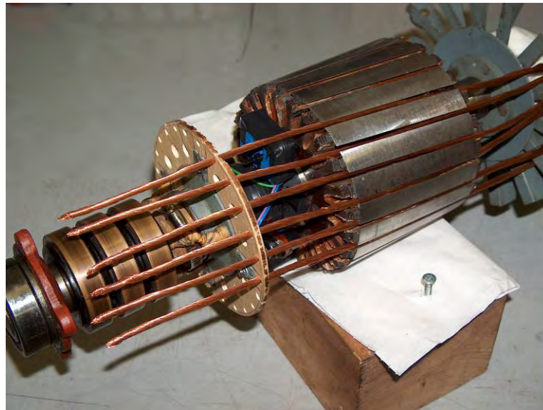
Fig.5.16. Construction of the improved cage.
