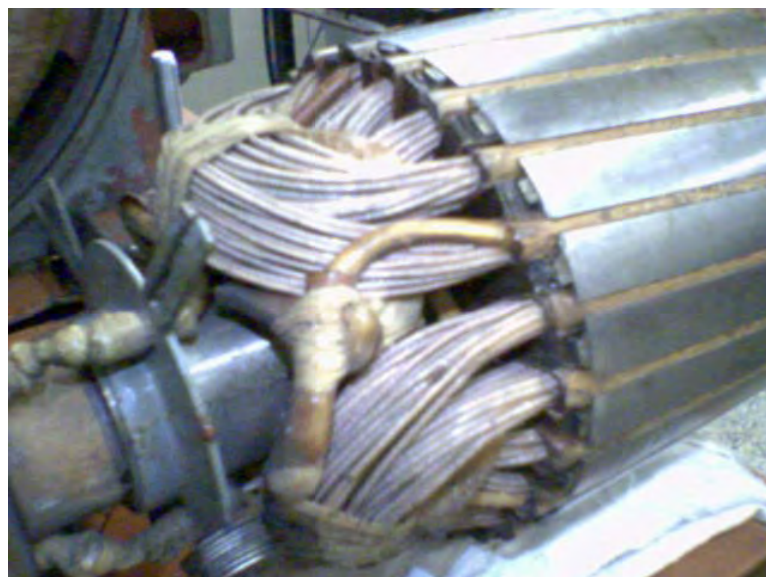
Fig.5.2. The three-phase rotor winding (with wood wedges).
