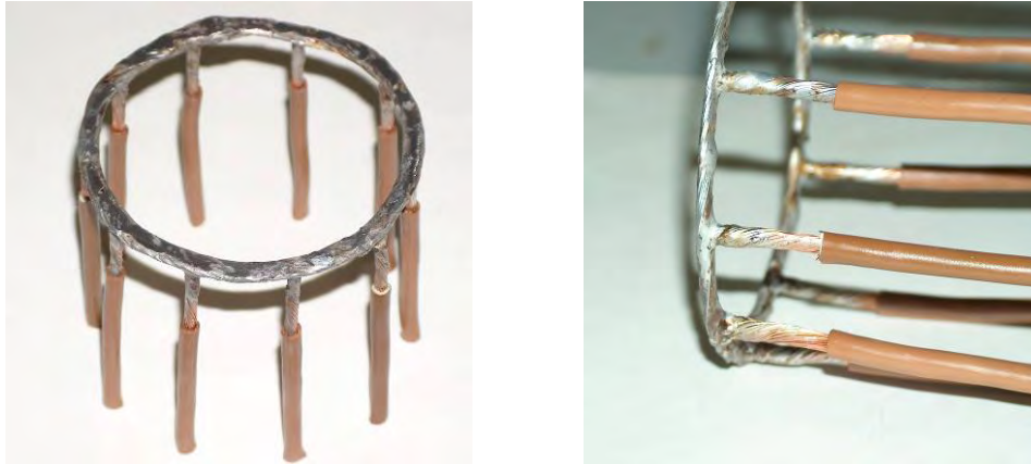
Fig.5.5. Direct-welded cage (prototype).
