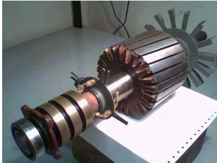
Fig.5.3. Nude rotor, 24 deep-slots, with possibility for single (thin or deep bars) or double cage allocation.
