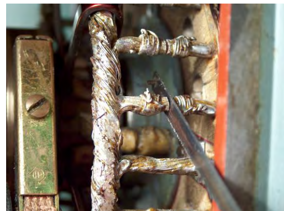
Fig.5.21. Left: the extremity of the cage is visible and easily accessible. Right: bar cutting. The bar can be completely repaired and interrupted again more and more times.
