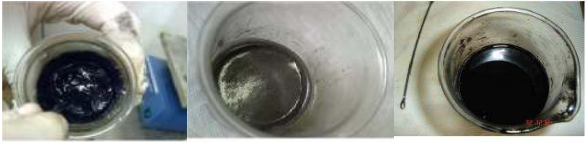
Fig.1.31. CNT-reinforced Epoxy-based composite sample preparation: viscosity lowering and air voids removal by means of ultrasonication methods.
