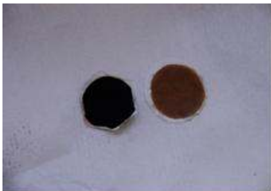
Fig.1.23. CNT functionalization procedure: vacuum-assisted filtration step. PTFE- 0.45\mu\text{m} and GV- 0.22\mu\text{m} porous membranes were employed to recovery the treated CNTs after the oxidation in acidic environment. The different colouring of both the solutions and the membranes stress the further purification/homogenization of the CNT material after the different stages of the filtration procedure.
