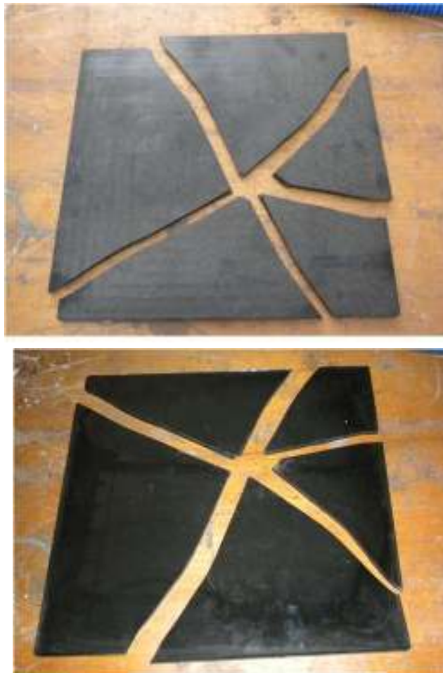
Fig.3.9. Ductile behavior of the NH 2 -MWCNT reinforced composite materials during the high energy ballistic CG test (up: front side; down: back side).
