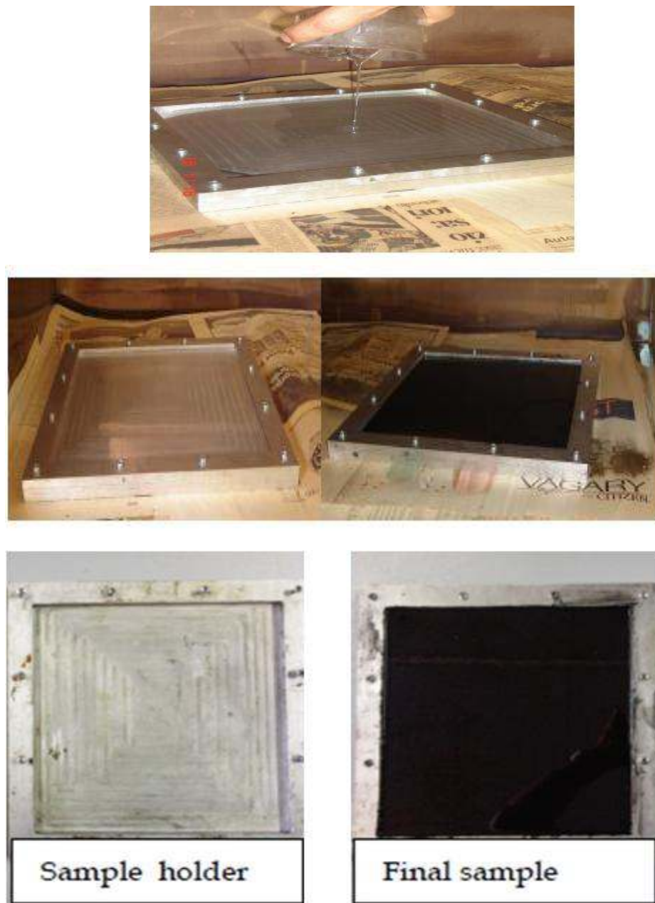
Fig.1.30. CNT-reinforced Epoxy-based composite sample preparation: pure and CNT-filled Epoxy pouring into the Aluminum molds .
