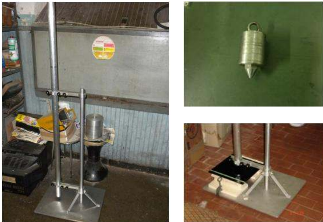
Fig.3.3. Picture of the in-house built dropped weigh tower system for the low energy ballistic characterization. On the left, the whole apparatus; on the right, the 0.5kg weight adopted (above), and the sample positioning (below).
