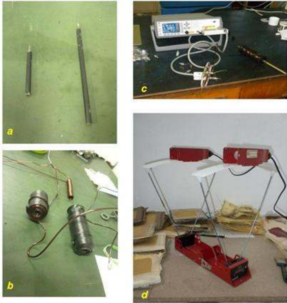
Fig.2.13. CG set-up pictures: a) short (S) and long (L) iron bullets; b) different copper coils tested; C) inductance static measurements by Agilent LCR Meters; d) ballistic ProChrono chronograph for bullet's speed measurements.
