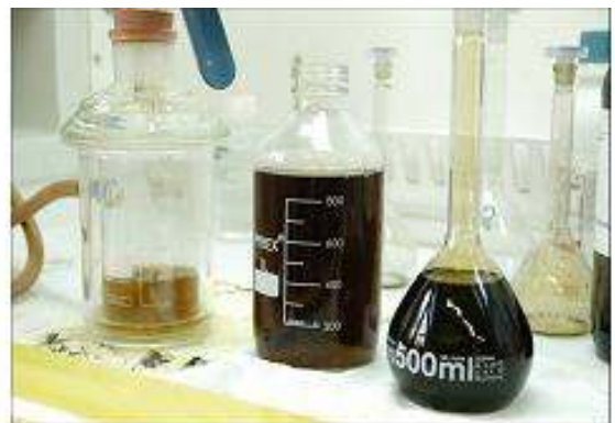
Fig.1.23. CNT functionalization procedure: vacuum-assisted filtration step. PTFE- 0.45\mu\text{m} and GV- 0.22\mu\text{m} porous membranes were employed to recovery the treated CNTs after the oxidation in acidic environment. The different colouring of both the solutions and the membranes stress the further purification/homogenization of the CNT material after the different stages of the filtration procedure.
