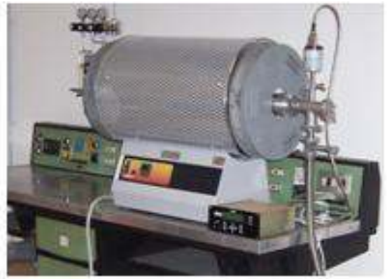
Fig.1.22. CNT functionalization procedure: in air oxidation step. A CVD oven (right) was utilized to remove impurities and amorphous carbon material from the as-received CNTs at \sim 350^{\circ}\text{C} for \sim 2\text{h} . Ceramic holders (left) have been used in order to avoid any type of contamination during such treatment.
