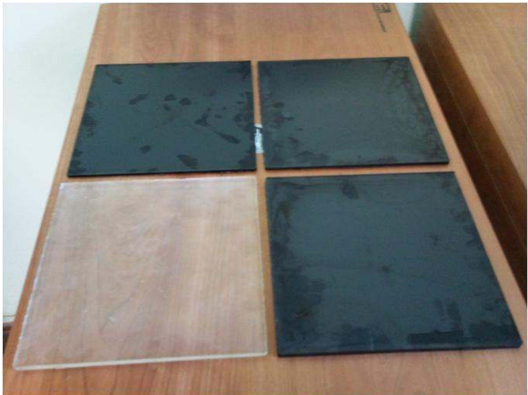
Fig.3.6. The four typologies of tile samples before the characterization by the Coil Gun facility: neat resin as not-reinforced reference samples, 0.5wt% micro graphite-reinforced, 0.5wt% pristine MWCNT-reinforced, and 0.5wt% amino-functionalized MWCNT-reinforced. Two reference thickness were defined for each kind of material typology: ~3mm and ~6.5mm.
