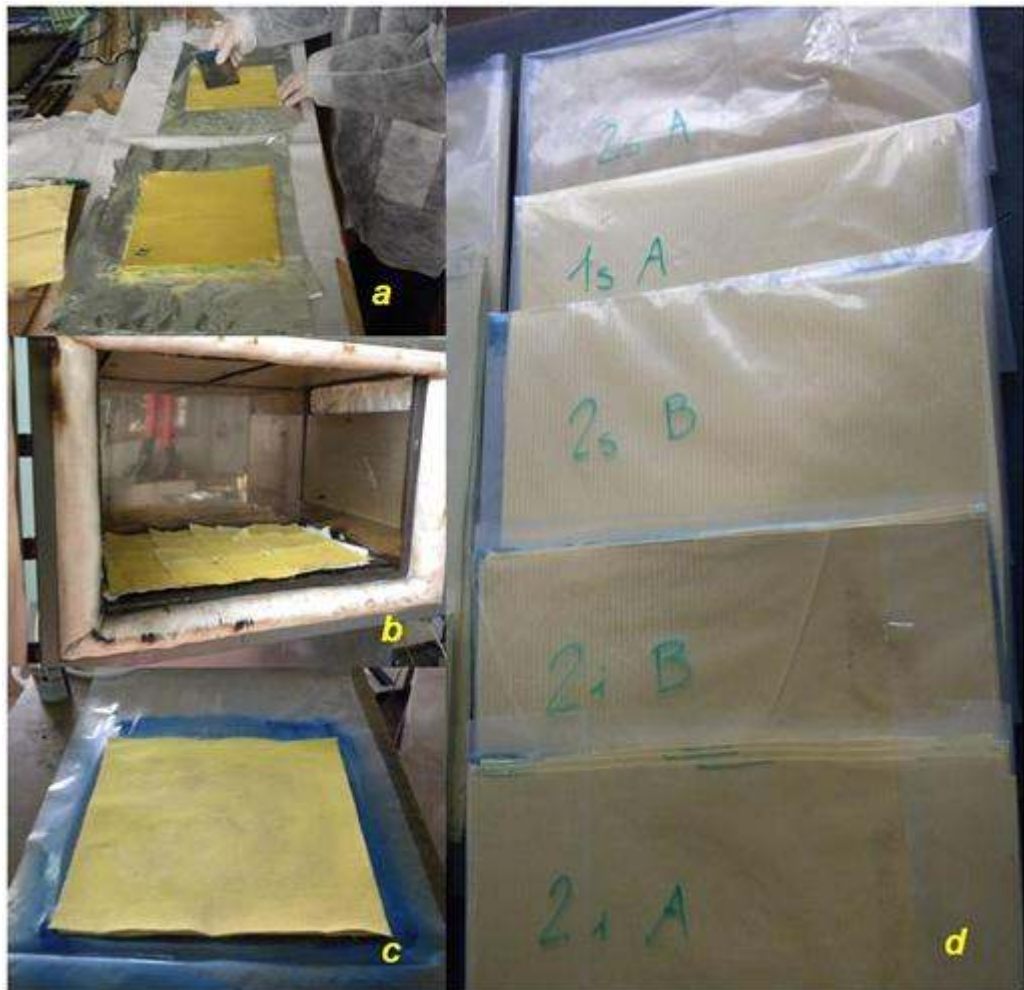
Fig.1.38. Different steps of Kevlar-reinforced based antiballistic panels manufacturing: a) fluid application onto layers surface, b) solvent evaporation in oven, c) enveloping procedure, d) the panels ready for the ballistic test.
